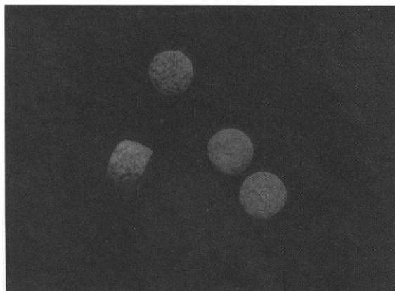
Fig. 5. Tablets after dissolution showing porous structure with intact tablet.
